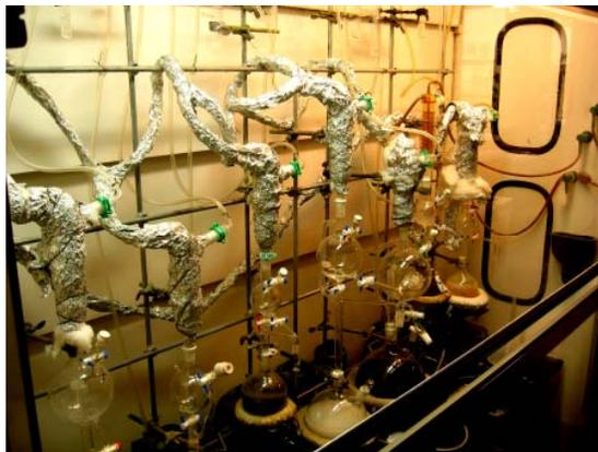
This job consists of taking care of the distillation of common solvents for the group. Under the large hoods of both labs, you can find the stills for the following solvents:
